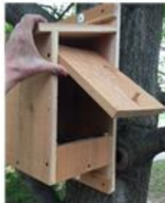
View of Door side with Door knob dowel, front hinge screw (front right top), protruding latching Pin (front right middle).
